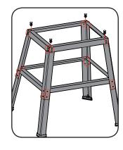
13 The Rubber Feet can now be fitted and the large bolts with rubber stops inserted into the rubber feet.
