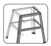
11 Align the holes of each opposing member. Bolts, washers and nuts can be inserted & tightened with hand force only.
