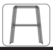
7 Align one short lower support inside the legs at the same height as the long lower support. Ensure that the lip of the side support is facing up.
