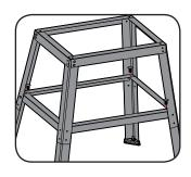
12 Once all of the members are joined together and all fasteners are assembled, place the 4 mounting bolts into the holes at the top of the stand. This will ensure the mounting holes align correctly while the stand is tightened.
