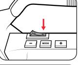
3 To remove, press and hold the battery release tab and pull the battery away from the tool.
