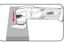
**Note:** Do not apply heavy pressure to the tool or tilt the sanding base as this will wear out the sanding paper and may damage the sanding pad.
