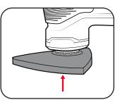
Press the sanding paper onto the sanding pad by aligning the edges and holes.
