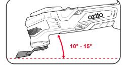
**Note:** Allow the scraper to do the work; do not apply heavy pressure to the tool. This may cause the multi function tool to overload or cut into the surface of the material.
