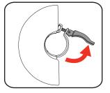
3 Tighten guard nut then close the guard lever.
