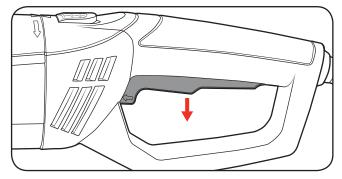
Note: The grinder is fitted with a soft-start switch for added safety.
