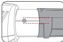
2. Rotate the blower nozzle to lock in place.
