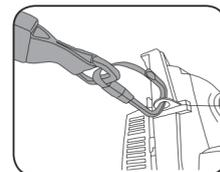
2. To unclip the jet blower, press either side of the buckle.
