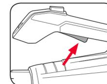
2. To stop operation, release the on/off trigger.
