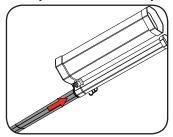
3. Secure the lower sections together with the supplied 45mm long assembly screw.
