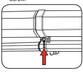
5. Slide the assembled tubes 6. Secure the tubes with the into the motor housing.
