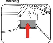
2. Attach the clip on the connector on the collection collection bag to the hook underneath the upper tube.
