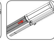
4. Slide the nose guide wheels over the lower tube and secure with the supplied 20mm long screw.
