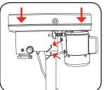
6. To fit the feed wheel handles, screw them into the feed wheel hub.
