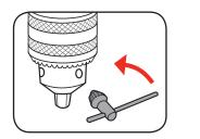
2. Insert the drill bit fully into the 13mm keyed chuck.
