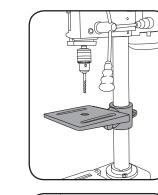
6. Slowly rotate the feed wheel handles to bring the drill bit down towards the table and into your workpiece. After drilling a hole, release the feed wheel handles slowly to return the 13mm keyed chuck to its original position.
