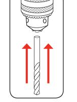
3. Whilst holding the drill bit in one hand, rotate the top collar of the 13mm keyed chuck in a clockwise Ensure that you tighten all 3 holes in the 13mm keyed chuck using the chuck key to securely tighten the jaws and hold the drill bit in position
