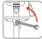
Loosen the table support angle bolt (located below the table) by rotating anticlockwise using an 18mm spanner or shifter (not supplied).
