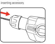
6. To remove the SDS-Plus accessory Try to pull it out. Note: It should have approximately 10 - 20mm movement This is normal.
