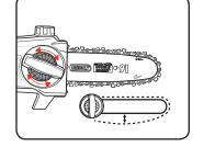
For the correct chain tension, firmly pull up on the chain at the middle of the top of the exposed guide bar. When the chain is pulled up to its highest point, the bottom tip of the links should only just stay in the track [middle of the guide bar]
