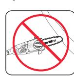
. Do not saw with the tip of the guide bar. This could lead to kick back and possible injury.
