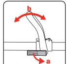
2. (a) Open the mounting bracket lever and (b) slide the auxiliary handle into the required position, close to lock into position.
