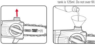
3. Refit cap and clean any oil spillage.
