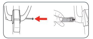
. Select the most comfortable position and close the lever to lock the auxiliary handle in
