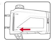
NEVER START WORK UNLESS THE CHAIN AND BAR ARE LUBRICATED
