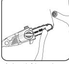
At the end of the cut, the weight of the pruner suddenly increases for the user, because it is no longer supported on the branch. There is the risk of losing control of the pruner.
