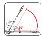
When removing branches, hold the pruner at an angle ranging from a maximum 60° to horizontal in order to avoid being struck by a falling branch.
