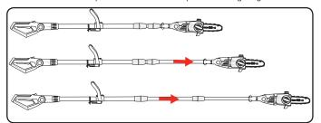
3. To lock in the desired position, twist the telescopic tube lock in a counterclockwise direction.
