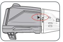
. (a) Press the pruner head against the motor head. This will cause the lock button to be pushed to the (b) Turn the pruner head
