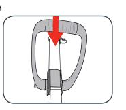
2. Pass the bolt through the auxiliary handle and screw the lever to the end
