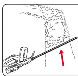
**WARNING!** IF THE BLADE JAMS ON ANY ELECTRICAL CORD OR LINE, DO NOT TOUCH THE BLADE! IT CAN BECOME ELECTRICALLY LIVE AND VERY DANGEROUS. CONTINUE TO HOLD THE HEDGE TRIMMER BY THE INSULATED REAR HANDLE OR LAY IT DOWN AND AWAY FROM YOU IN A SAFE MANNER. DISCONNECT THE ELECTRICAL SERVICE TO THE DAMAGED LINE OR CORD BEFORE ATTEMPTING TO FREE THE BLADE. FAILURE TO HEED THIS WARNING MAY RESULT IN SERIOUS PERSONAL INJURY OR POSSIBLE DEATH.
