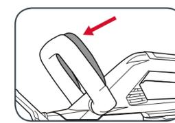
2. To start the hedge trimmer, squeeze the on/off trigger.
