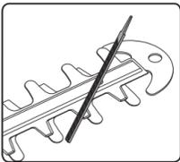
4. Remove the hedge trimmer from the vise and insert the battery pack. Repeat steps 1-3 for the unsharpened edges of the blade teeth.
