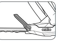
WARNING: NEVER USE THE HEDGE TRIMMING UNLESS THE SAFETY GUARD IS FITTED.
