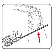
IF THE BLADE JAMS ON ANY ELECTRICAL CORD OR LINE, DO NOT TOUCH THE BLADE! IT CAN BECOME ELECTRICALLY LIVE AND VERY DANGEROUS. CONTINUE TO HOLD THE HEDGE TRIMMER BY THE INSULATED REAR HANDLE OR LAY IT DOWN AND AWAY FROM YOU IN A SAFE MANNER. DISCONNECT THE ELECTRICAL SERVICE TO THE DAMAGED LINE OR CORD BEFORE ATTEMPTING TO FREE THE BLADE. FAILURE TO HEED THIS WARNING MAY RESULT IN SERIOUS PERSONAL **INJURY OR POSSIBLE DEATH.**
