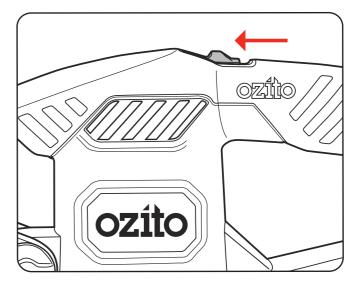
2. To turn the sander off, slide the on/off switch backward.
