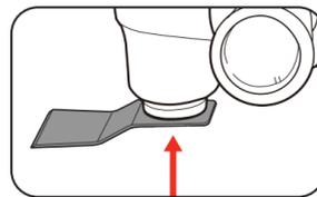
**Note:** Ensure the accessory is sitting flat on spindle and locking pins.
