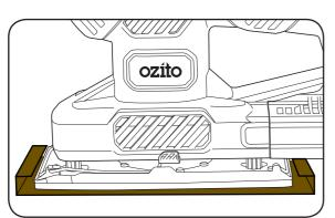
3. Feed the paper under the paper clip at the front of the sander. Lock the clamp.
