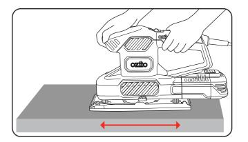
Note: Keep the entire sanding pad in contact with the workpiece at all times during sanding.
