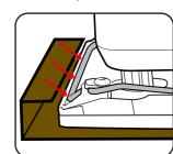
4. Feed the paper under the paper clip at the rear of the sander. Lock the clamp.
