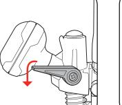
To release the plunge lock mechanism, pull the lever up.
