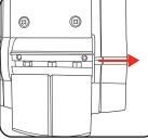
1. Loosen the 3 hex head screws using the spanner provided.
