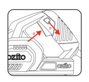
3. Release on/off switch to turn off.
