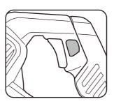
2. Depress the lock-on button and then release the on/off
