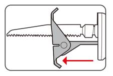
3. Push the locking button back to the right to lock the pivot shoes position.
