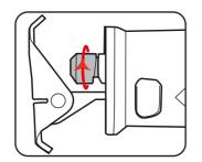
2. Insert the blade through the pivot shoe and into the blade holder.
