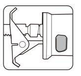
2. Reposition the pivot shoe to the desired position.
