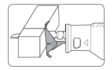
DO NOT ALLOW THE TOOL TO BOUNCE. IF THE PIVOT SHOE IS HELD AWAY FROM THE WORK PIECE DURING OPERATION, STRONG VIBRATION AND/OR TWISTING MAY OCCUR CAUSING THE BLADE TO SNAP DANGEROUSLY.
