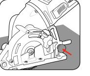
2 Lower the circular saw body, plunging the blade into the work piece.
