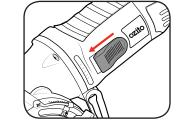
4 Press the plunge release button and lower the blade into the work piece.
