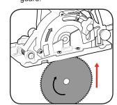
Note: Before starting the saw, ensure that the blade is fitted correctly and moves smoothly.
