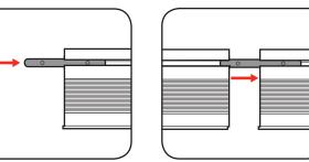
3 Secure the guide rails together by tightening the 2 hex screws.
