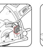
3 Secure the cutting depth by tightening the depth locking screw.
