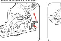
Replace the blade, ensuring the blade direction matches the arrow on the
