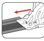
2 Position the guide rail so that the edge of the rail rests against the marked line.
