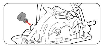
2 You can now connect a suitable vacuum or dust extractor to the other end of the adaptor.
