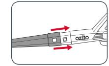
3. To remove the blower tube, press the blower tube release tab while pulling the tube away from the housing.
