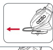
Align the tabs of the safety guard with the recess in the back of the cutter head.
