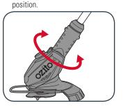
Rotate the head into the desired
