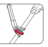
Rotate the handle into the desired position and then lock in place with the lever.
