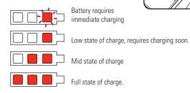
**Note:** The battery needs to be removed from the tool to check the state of charge.
