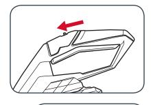
2. Squeeze the on/off trigger to start the trimmer.
