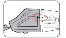
(a) Press the trimmer head against the motor head. This will cause the lock button to be pushed to the (b) Turn the trimmer head
