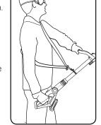
Trimming new growth Using a wide sweeping motion. feed the blade teeth through the twigs. A slight downward tilt of the blade, in the direction of motion gives the best cut.
