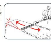
**Note:** Do not use the pole hedge trimmer for cutting stems greater than 12mm. Use the trimmer only for cutting normal shrubbery found around houses and buildings.
