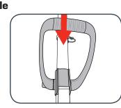
2. Pass the bolt through the auxiliary handle and screw the lever to the end
