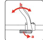
2. (a) Open the mounting bracket lever and (b) slide the additional handle into the required position, close to lock into position.
