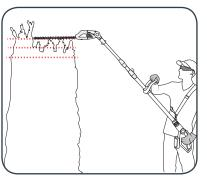
• General information. When older hedges are to be cut back a substantial amount, use pruning shears or some other device to trim thicker branches (greater than 12mm diameter) to the desired length before starting work with the pole hedge trimmer. Ensure the blades do not come into contact with any object made of hard material that could damage the blades, such as wire fencing or metal plant supports.
