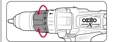
**Note:** Selecting a higher torque setting will allow the drill to use more torque to drive the screw in or out. To prevent damaging the screw head, it is recommended to start at a low torque setting and increase when necessary.
