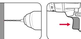
6 Move the drill bit into the workpiece.
