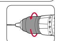
4 Pull on the bit to ensure it is firmly secured.
