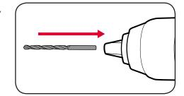
3 Tighten the chuck by turning
