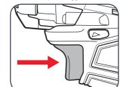
2 Release the variable speed trigger to stop the driver.
