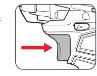
6 Slowly increase pressure on trigger to appropriate torque for circumstances until screw or bolt is tightened.
