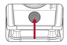
2 To turn the light off, press the on/off switch
