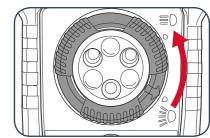
2 For a wide beam, rotate the beam setting dial clockwise "
