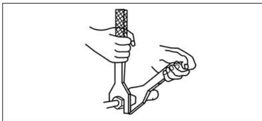
Ø 6 mm Rohr = 15 - 20 Nm
