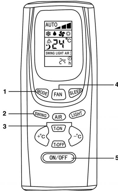
The temperature can be set from 16°C to 30°C on the remote control via the "Cooling", "Dehumidifying" and "Heating" operating modes.
