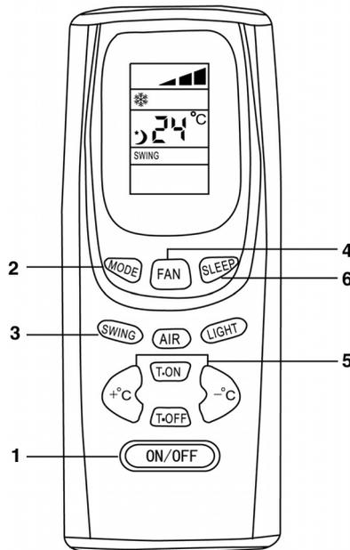
**E) Timer settings (for automatically switching the device on/off)****1. "T-ON" (device ON timer) key**
