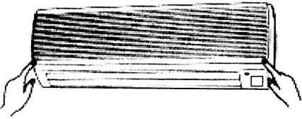
Pull on the bottom corners of the intake grille. The grille will swing up (approx. 25°) and will stay in this position.
