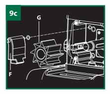
Clean the cutting compartment, the counter blade and the cutting unit and cover them with a thin coat of vegetable oil before installing everything again. At the beginning of the new season the counter blade must be correctly adjusted as described on page 25.
