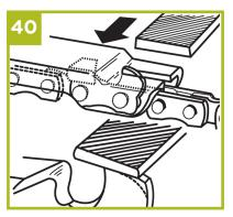
After sharpening, the cutting links must all have the same width and length.
