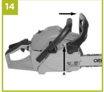
**Note:** The brake lever should snap into both positions. If strong resistance is felt, or lever does not move into either position, do not use your saw. Take it immediately to a professional Service Center for repair.
