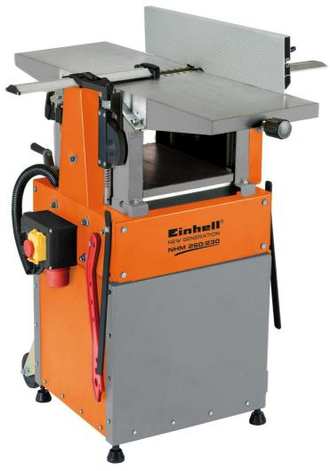
The NHM 260/230 surfacing and thicknessing plane is designed for high standards of accuracy and precision within its working range. Universal machining options include the squaring and truing up of rough timber or planing to exact thickness on the thicknessing table. The joint stop is horizontally adjustable and can be tilted through 45°for chamfering. The knife shaft is equipped with two reversible planing knives for high performance – maximum chip depth 3 mm – and optimum, fine surfaces.
