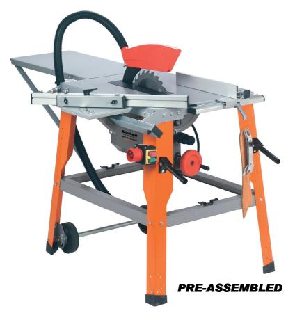
The BK 315/400 circular bench saw is powered by a strong 2,2 kW induction motor with mechanical brake. The saw is powder-coated and therefore permanently protected against corrosion. The ball-raced height adjustment permits easy and precise setting of the saw blade.
