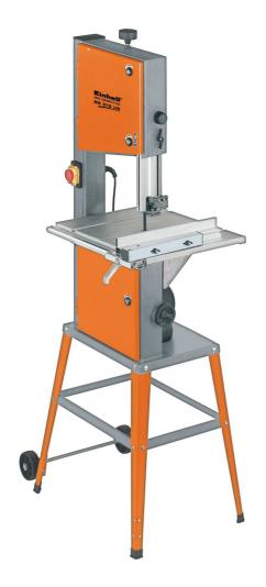
The powerful BS 315 UG band saw offers many precision-cutting options, e.g. longitudinal cuts, mitre cuts or freehand cuts. The band saw is ideal for cutting wood, plastics or similar materials. The pin guide ensures optimum guidance of the band saw blade. In addition, the BS 315 UG is equipped with an adapter for connection of a dust extractor.
