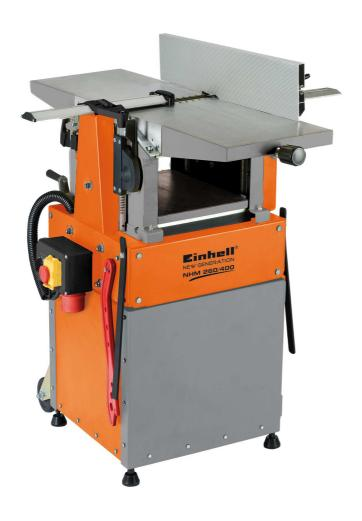
The NHM 260/400 surfacing and thicknessing plane is designed for high standards of accuracy and precision within its working range. Universal machining options include the squaring and truing up of rough timber or planing to exact thickness on the thicknessing table. The joint stop is horizontally adjustable and can be tilted through 45° for chamfering. The knife shaft is equipped with two reversible planing knives for high
