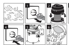
For dry-vacuuming, slip the pleated filter (Figure 2) onto the filter basket.
