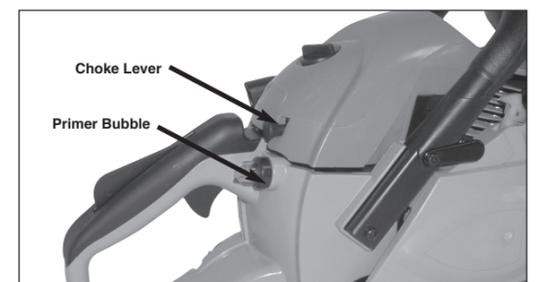
**NOTE: amount of choke will vary slightly Depending on the external temperature (Warm = choke OFF, cold = Choke ON)**
