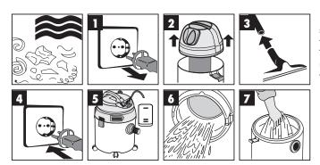
For wet-vacuuming, slip the supplied foamed plastic filter over the filter basket (Figure 2). The pleated filter already fitted upon delivery is not suitable for wet-vacuuming!
