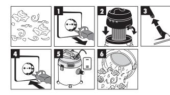
For dry-vacuuming, slip the pleated filter (Figure 2) onto the filter basket
