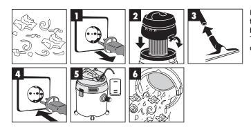
For dry-vacuuming, slip the pleated filter (Figure 2) onto the filter basket. The pleated filter is suitable for dry-vacuuming only.
