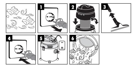
For dry-vacuuming, slip the pleated filter (Figure 2) onto the filter basket.
