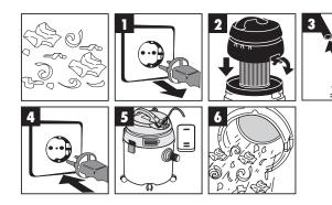
For dry-vacuuming, slip the pleated filter (Figure 2) onto the filter basket
