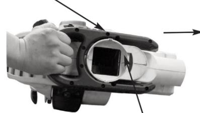
Ensure connecting tube is fitted correctly in housing and engages safety cut out switch.
