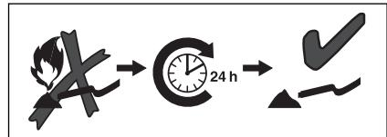
Wait at least 24 hours before vacuuming an oven or a fireplace in order to be sure that the fire has gone out and the ash has cooled down. Only for cold ash, see the operating instructions!
